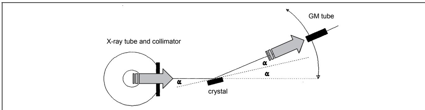
The GM tube is mounted on a rotatable measuring arm. The rotations of the crystal and the GM tube are coupled: to rotate the crystal over an angle  $\alpha$ , the GM tube has to be rotated over an angle of  $2 \cdot \alpha$ . As a consequence, the GM-tube always measures the intensity of the X rays reflected by the lattice planes of the crystal (see the diagram above).
