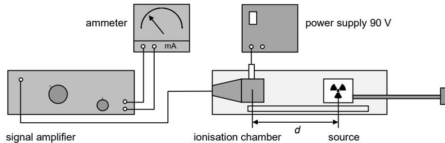
With the equipment set-up, the range  $R$  of  $\alpha$  particles in air can be determined by measuring the ionisation current  $I$  as a function of the distance  $d$  between source and ionisation chamber.
