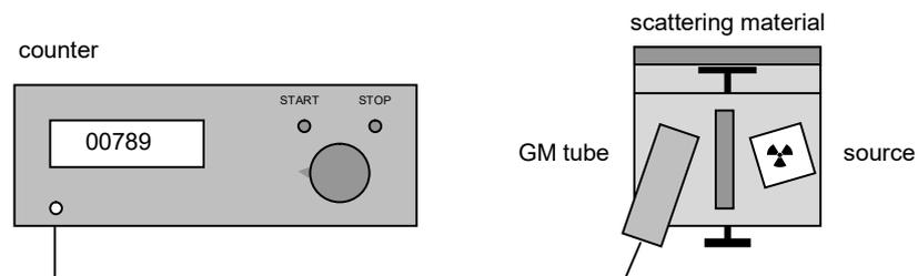
With the equipment set-up, the intensity  $I$  (in pulses per unit of time) of the back-scattered  $\beta$  radiation can be measured for different scattering materials: carbon, iron, aluminium, copper, tin and lead – and an unknown material.
