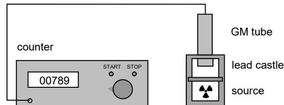
With the equipment set-up, the intensity  $I$  (in pulses per unit of time) of the transmitted  $\beta$  radiation can be measured as a function of the thickness  $d$  of the absorbing material.
