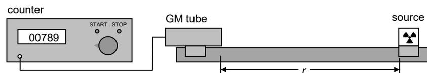
With the equipment set-up, the radiation intensity  $I$  (in pulses per unit of time) can be measured as a function of the distance  $r$  between the source and the GM tube.
